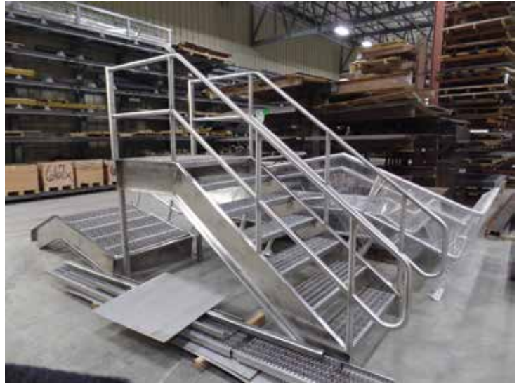
Stainless Steel Platform and Railings
